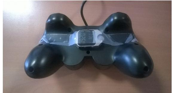
Figure 2. The gamepad and the accelerometer.
